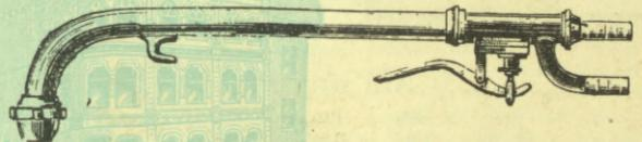
No. 276. Fitted with self-acting and regulating valves and continuous lighting jet. By releasing lever gas valve closes. Quantity of gas consumed can be regulated to suit description of work to be brazed. Each, \$7.50.
