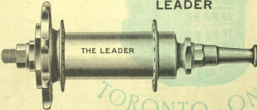
No. 998. "Leader" made from bar steel, cups and cones turned from special cone steel, accurately ground, chain line  $1\frac{1}{2}$ " or  $1\frac{5}{8}$ ", sprockets 7 to 12 tooth for  $\frac{3}{16}$ " chain.
