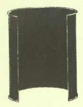
"Treasure Oak" Bodies are made of one piece Heavy Superior Cold Rolled Steel and Flanged Top and Bottom. In mounting, the body is forced over a flange on top of Fire-Pot into cement filled cup joint. Body flange is then turned, and over this Deflector Ring is bolted, making an absolutely air-tight joint, which cannot open or leak.
