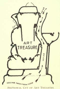
Showing construction and how the cold air is taken from the floor, heated and passed out the top, where it is distributed to all parts of the room. The upper end of the flue is supplied with a Pipe Collar, to which a pipe may be attached for conveying hot air to rooms above. This Flue is equal in capacity to an eight-inch Hot Air Pipe.
