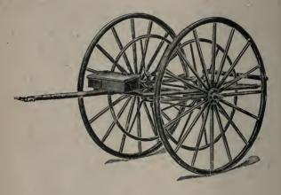
These carts are made in three sizes, intended for use in places where only a small quantity of hose is required. They are substantially built, and cap able of withstanding rough usage. The frame and reel are made of tubular steel, and the wheels are wood. They have tool box in front and friction roller at rear. Neatly painted and striped.
