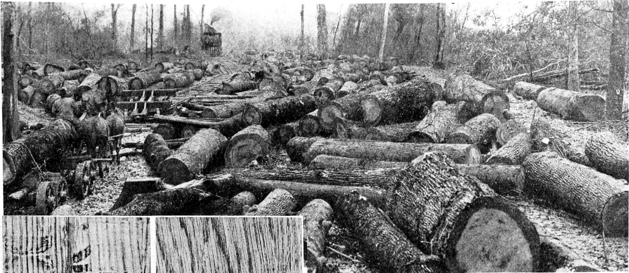
These Are the Logs That Make the Lumber That Makes the Trim, the Floors and Furniture of the Homes We Live in. Some of the Logs Will be Sawed Parallel to The Radii, to What are Known as Medullary Rays, Producing a Flake in the Grain—Quartered Oak.
