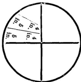
**HEADING BOLTS** are generally made of sound Bass-Wood, or Whitewood, timber either 18 inches long or 37 inches, and not less than 8 inches in diameter. If from 8 to 12 inches in diameter, leave them whole ; if from 12 to 18 inches, halve them ; if over 18 inches, quarter.
