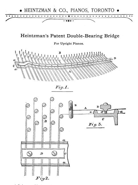
A, Strings. a, Ringing Points. B, Tuning Pins. C, Bridge. D, Bearing Bar. d, Ringing Point.
