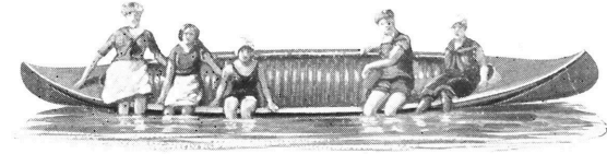
The "SPONSONS" support the weight and keep the gunwale above water.
