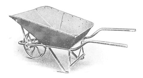
No. 331—Steel Coal Barrow. Made in sizes to carry from 250 to 500 lbs. coal. It is balanced so that the load is over the wheel. Prices on request.
